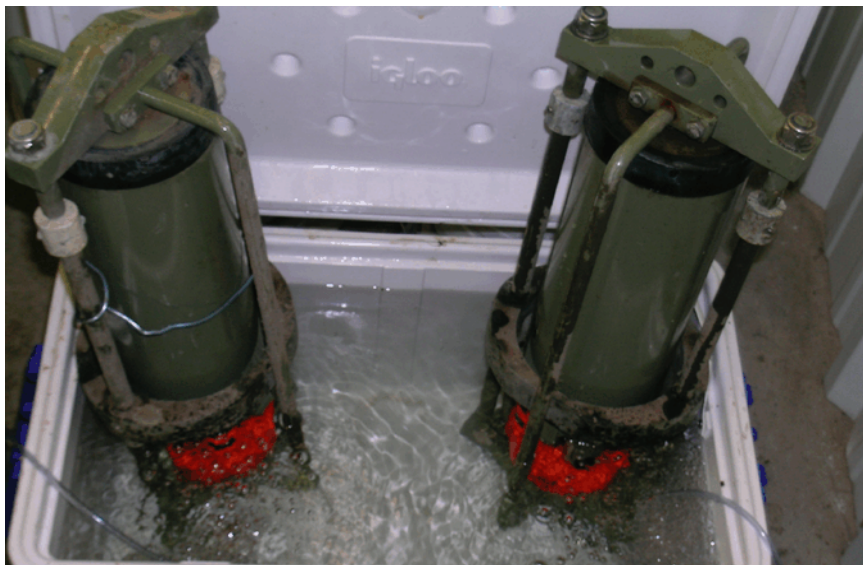
Figure 6-3. Cleaned and Reconditioned Mk II with Optode 3830 in Storage Tank Used Between Deployments
