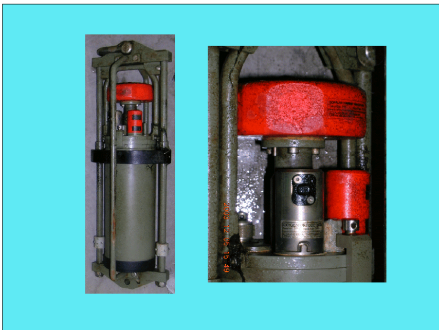
Figure 6-4. Mk II with Optode 3830 After Freshwater Deployment, with Close-up of Mk II with Optode 3830 (right)
