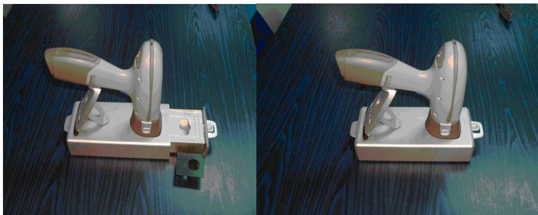
Figure 3-1. XLt with open sample drawer (left) and with closed sample drawer (right), ready for analysis.
