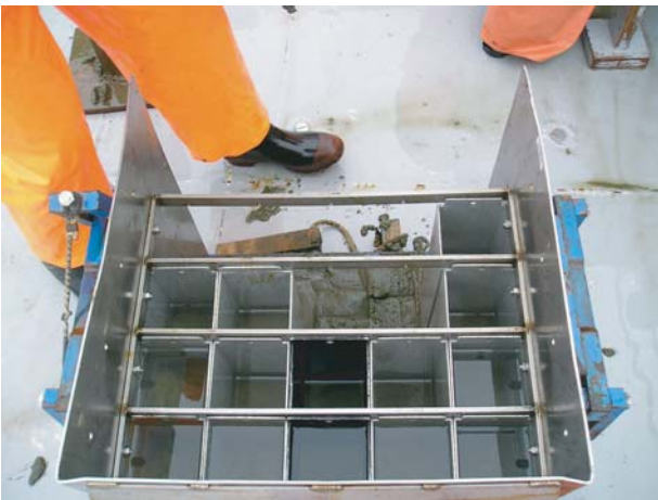
Some of the subcores have been removed for chemistry and biology samples.
