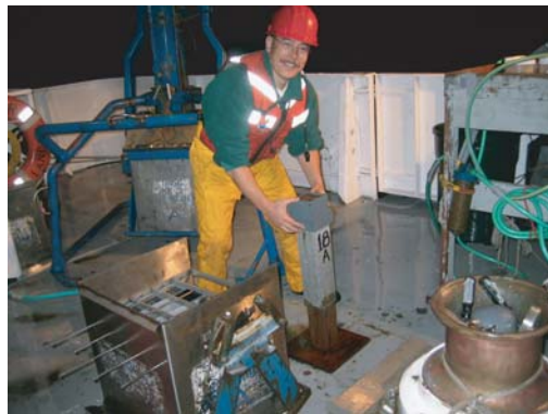
Sediment being extruded for processing from one of the subcores.
