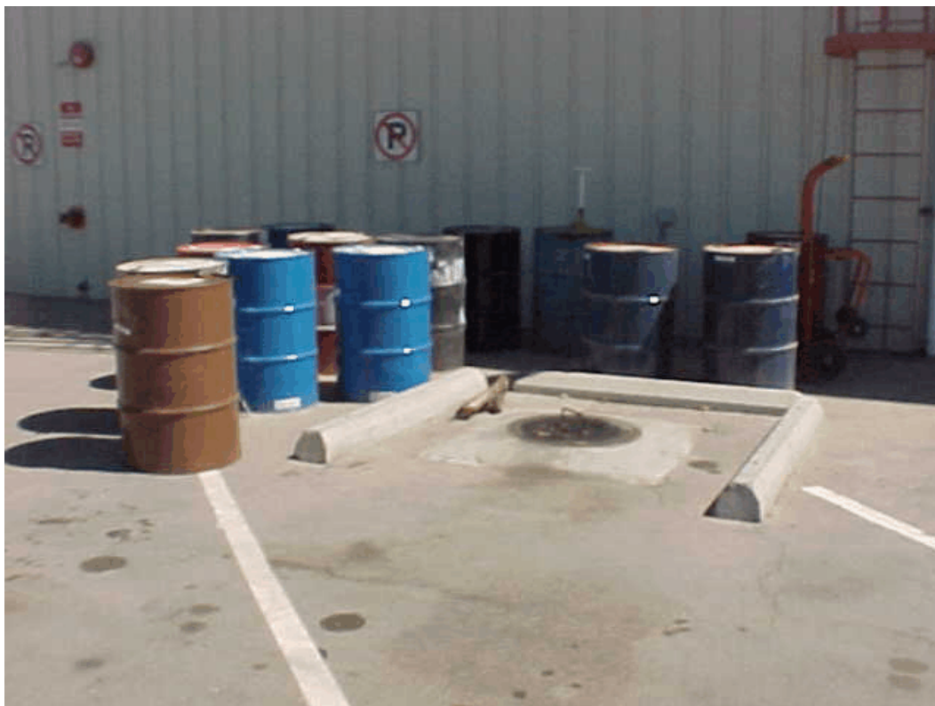
Photo 4. Waste oil pit and multiple 55-gallon drums that are full, partially full, and empty at the Automotive Repair facility.
