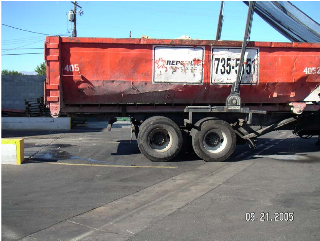
Photo 1. Roll-off container is leaking.
