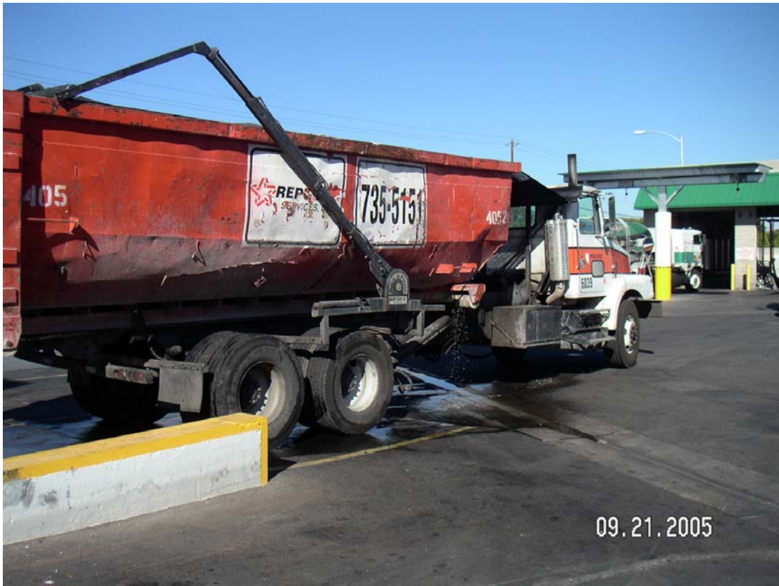
Photo 3. Roll-off container is leaking.
