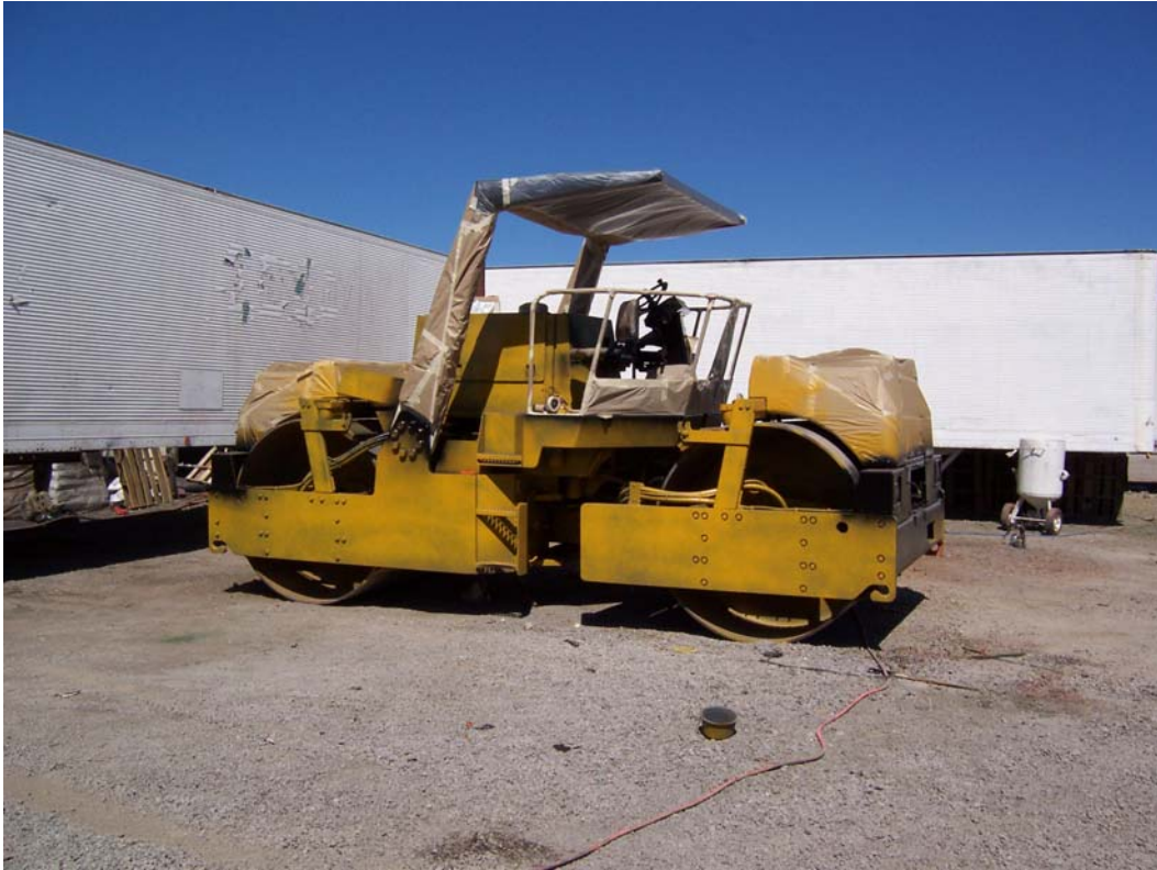
Photo 2. Roller masked for open air spray painting operation.
