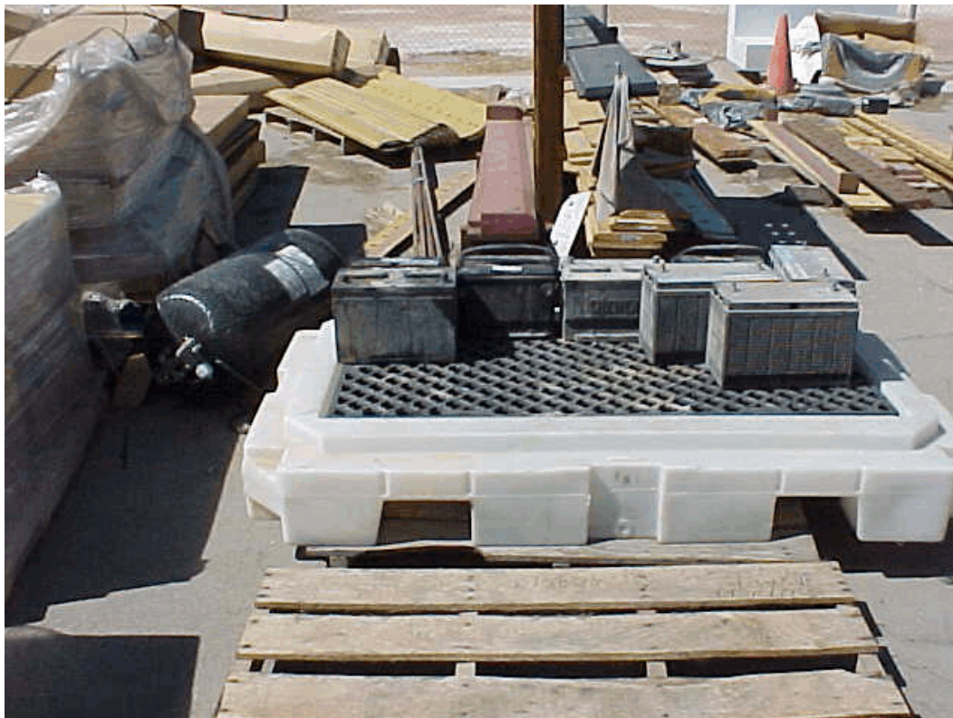
Photo 3. Exposed, but contained used batteries located outside the Automotive Repair facility.
