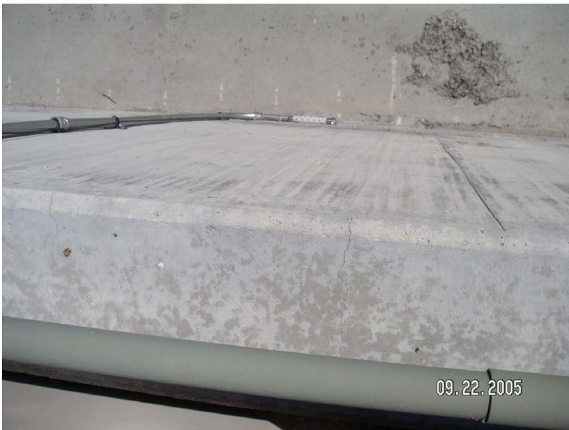
Photo 10. Meadows Detention Basin - influent sample probe about six inches from bottom of channel.
