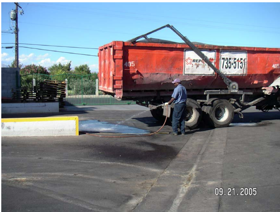
Photo 2. Roll-off container is leaking.
