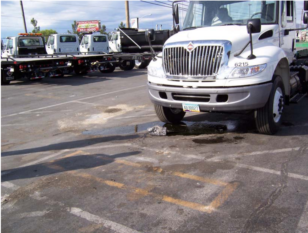
Photo 1. Oil leaking from truck stored in the parking area.
