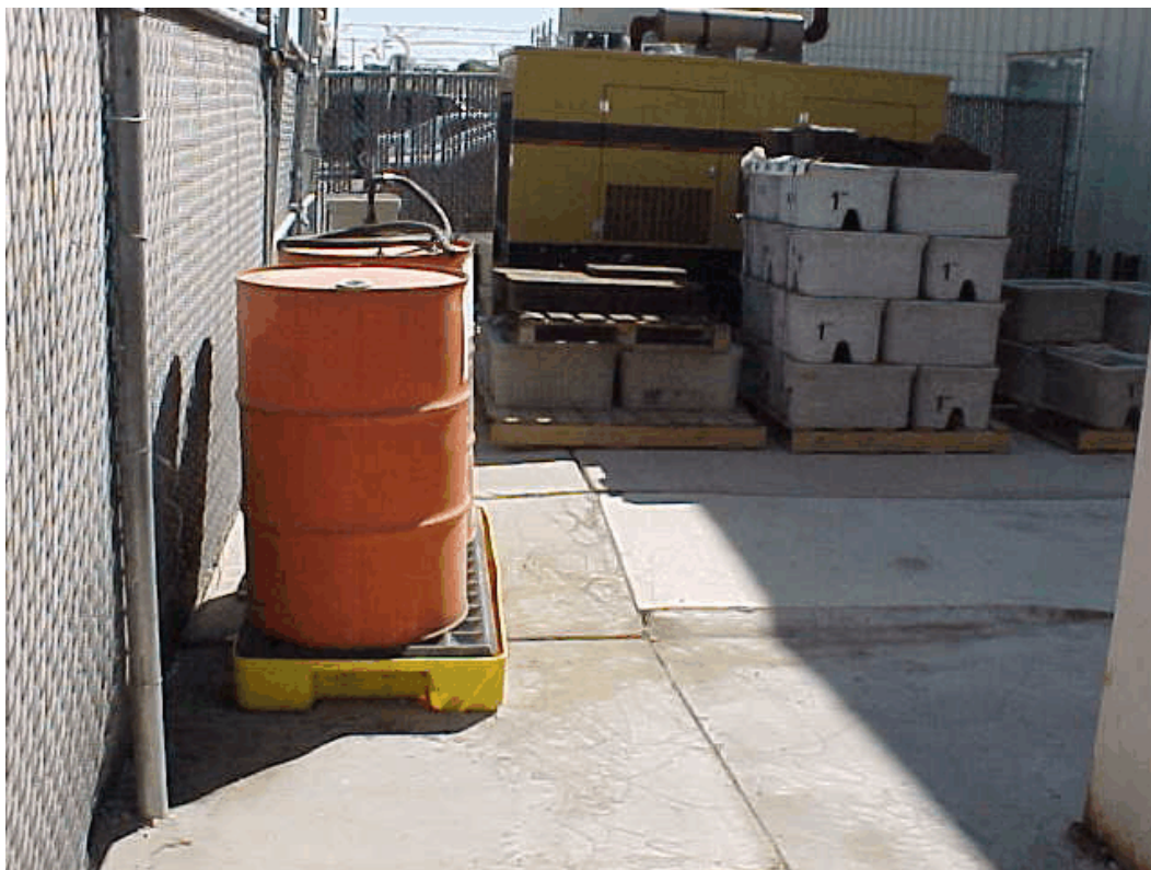
Photo 2. Fleet (primary) facility: Two uncovered 55-gallon drums of solvent.
