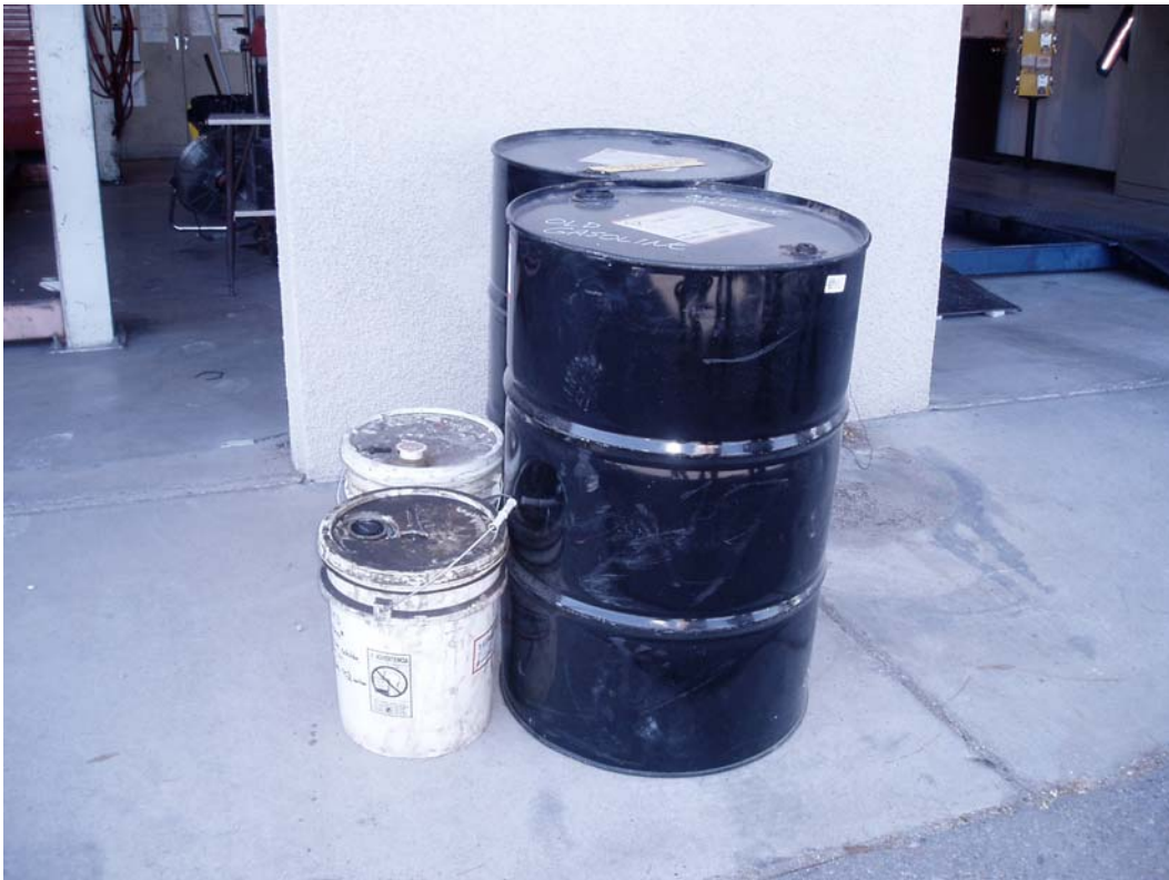
Photo 1. Two 55-gallon drums of used gasoline and two smaller buckets located outside the garage and without secondary containment.
