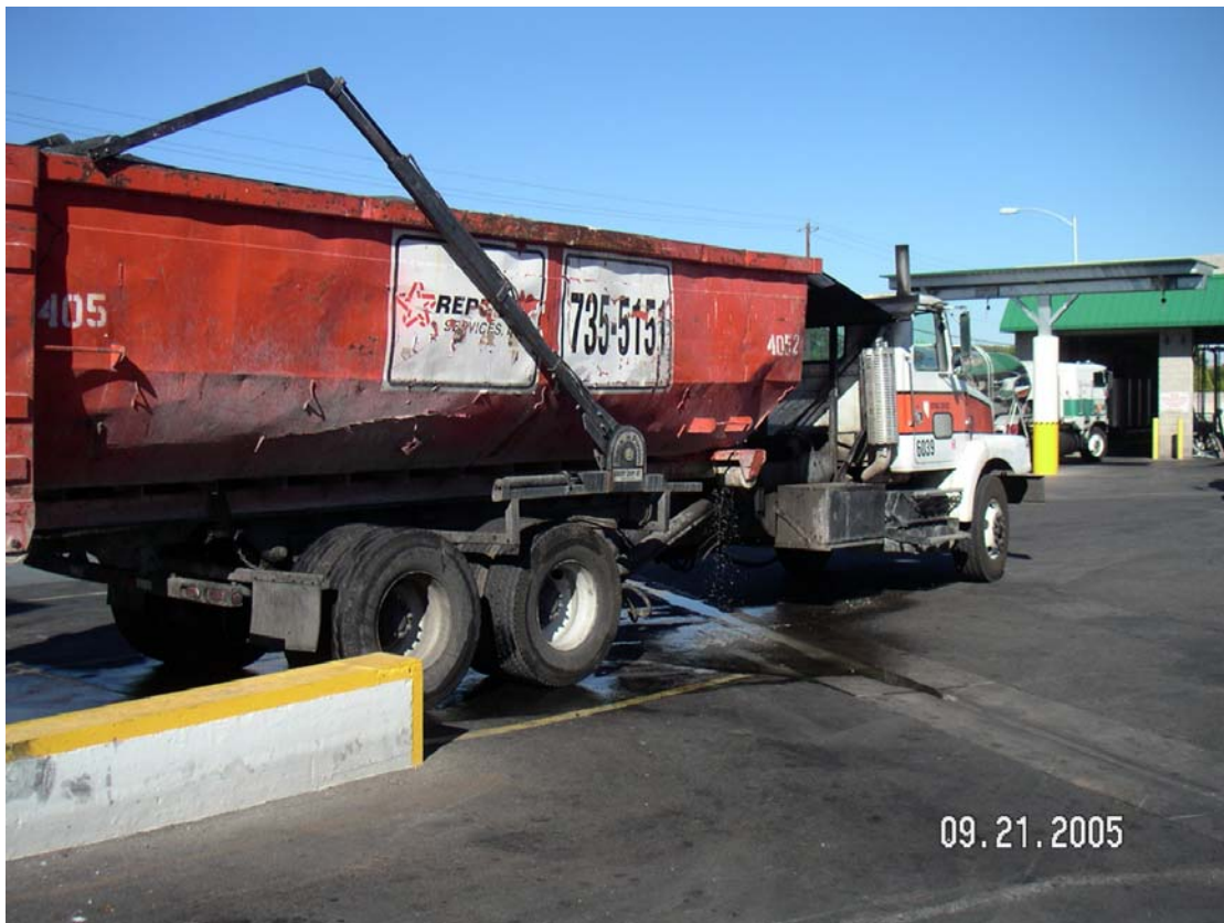
Photo 3. Roll-off container is leaking.
