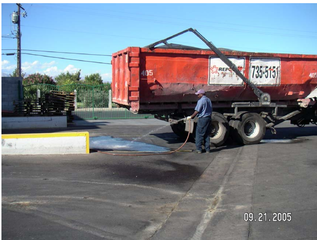
Photo 2. Roll-off container is leaking.
