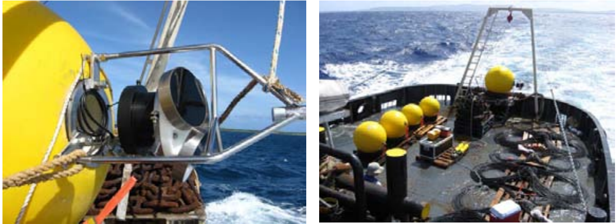
Figure 8. Deep Sea Current Meter Array Components: Float with Intergrated Mount for ADCP (left) and Components Waiting Deployment.
