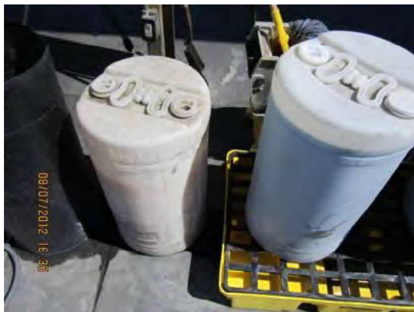
Photograph 5. View of drum of unlabeled container of fluid stored in an uncovered area without secondary containment adjacent to the vehicle wash bay shown in Photograph 4.
