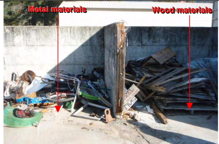
Photograph 10 – Storage area for materials picked up from the highways (Note: Area is uncovered and not bermed)
