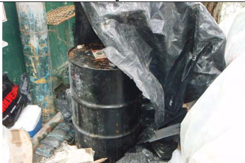
Photograph 8 – 55-gallon drum of “Rock Drill 150” that is partially covered and not within adequate secondary containment
