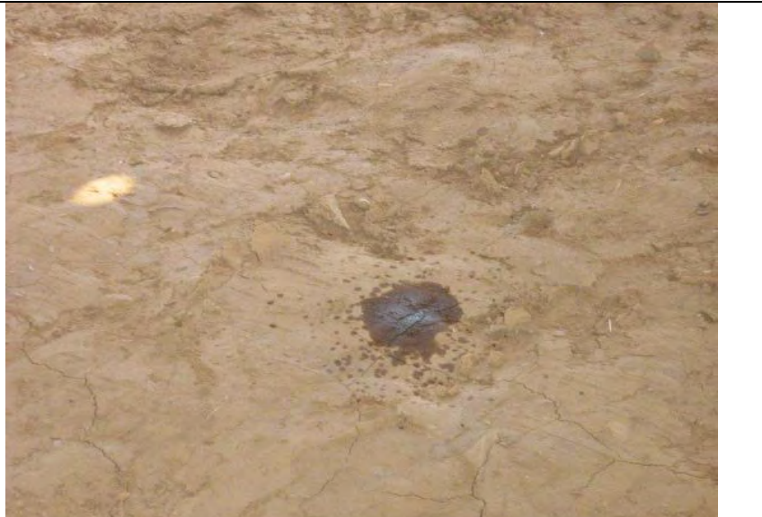
Photograph 4 – Close-up view of petroleum product on ground surface
