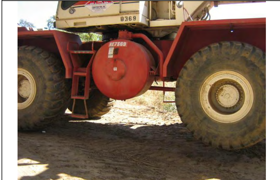
Photograph 3 – Equipment with petroleum product leaking onto ground surface (see Photograph 4 for close-up view).
