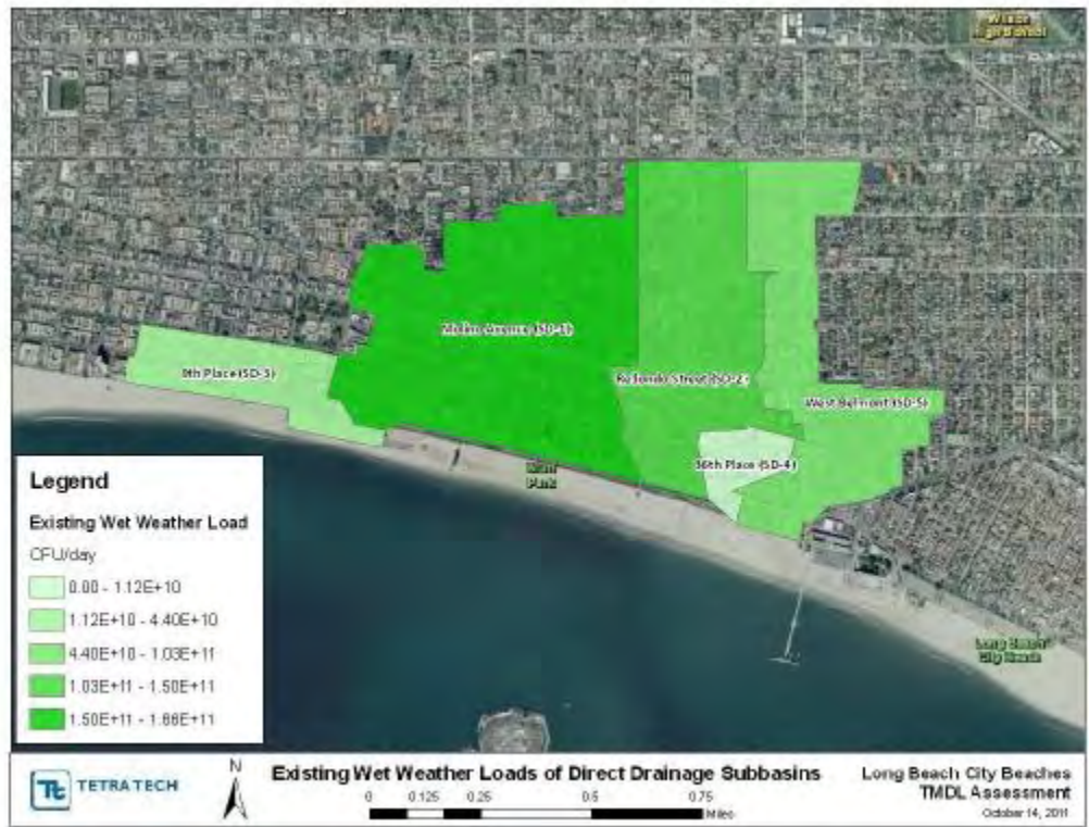
Figure 6-3. LBC beaches direct drainage wet weather loading
