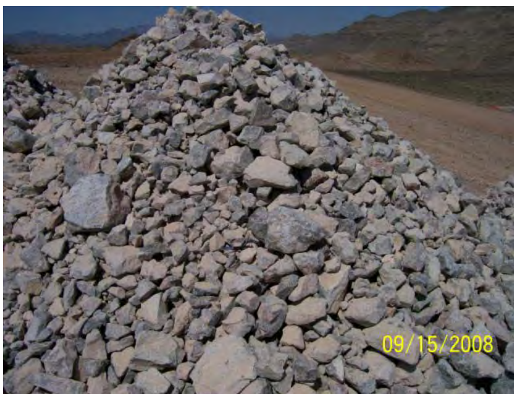
Photo 2 Erosion Layer Material
