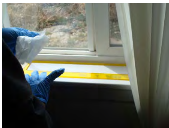
Tribal staff taking dust wipe sample at homes to determine potential lead hazards. Samples are sent for lab analysis. In pre-1978 housing, abrasion generates lead-contaminated dust from painted walls, floors, and window frames.
