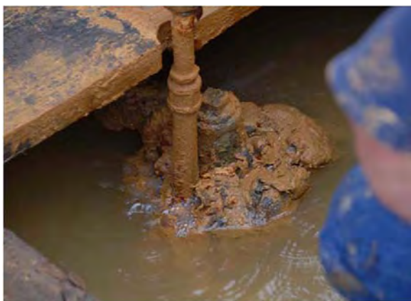
Top of well head encased in sludge precipitated from high TDS discharge.
