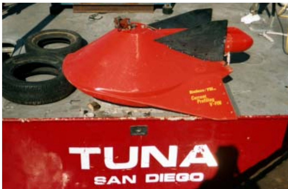
Figure 3-18. Acoustic Doppler Current Profiler (ADCP) towfish on deck of MV Tuna
