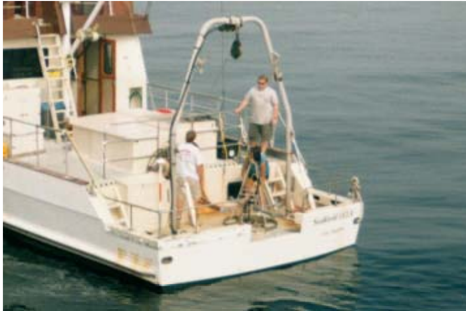
Figure 3-23. Video camera frame on deck of RV Sea World prior to deployment
