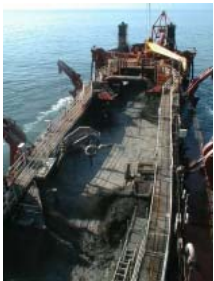
Figure 2-2. Photos of the hopper dredge Sugar Island , showing filling and cap placement operations
