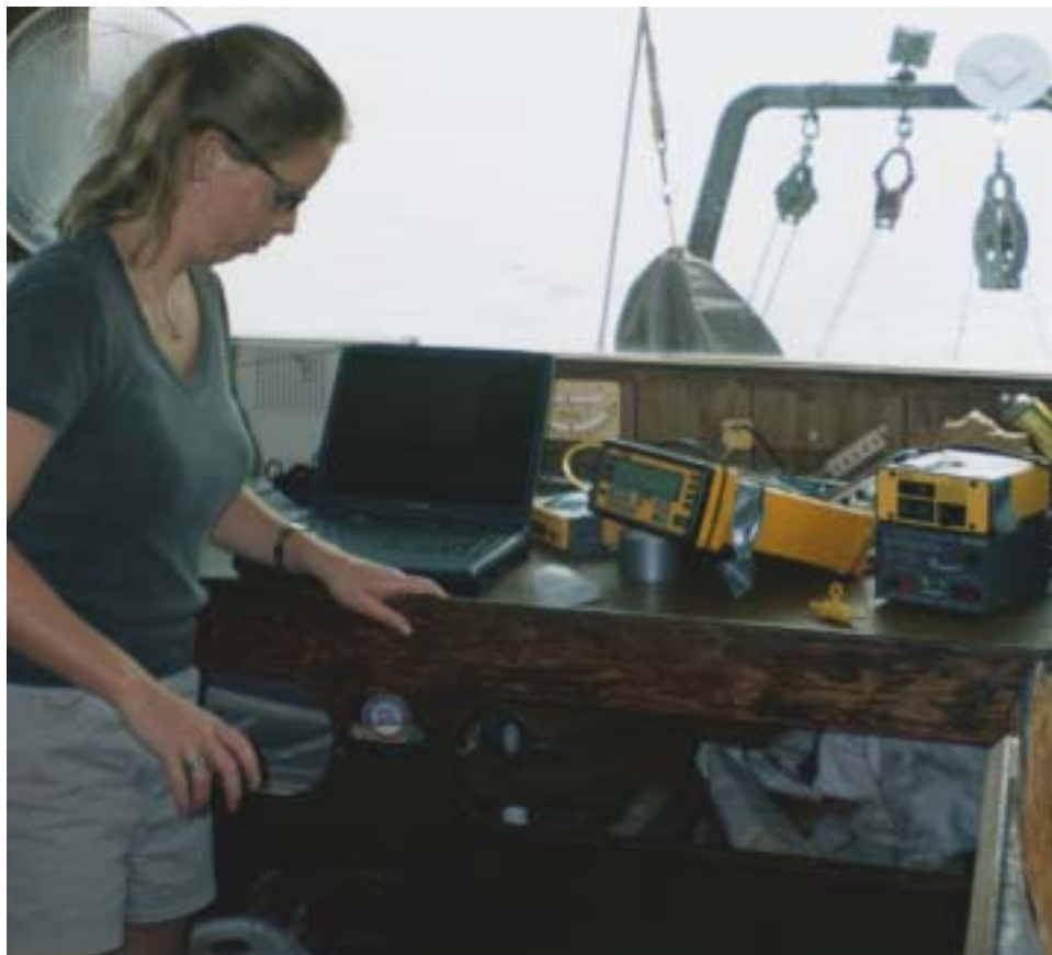
Figure 3-15. Navigator and DGPS navigation related equipment aboard one of survey vessels. The DGPS equipment was linked to laptop computer for visual real-time display of vessel position and target sample locations
