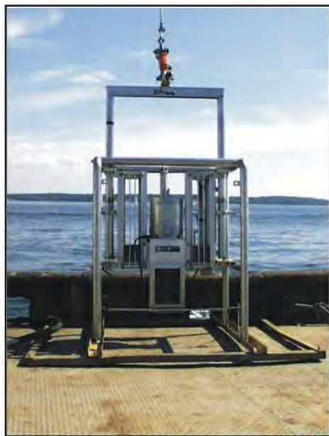
Figure 2.2-3. Schematic diagram of Benthos, Inc. Model 3731 REMOTS ® sediment-profile camera and sequence of operation on deployment. Photographs show sediment-profile camera with plan-view camera attached.
