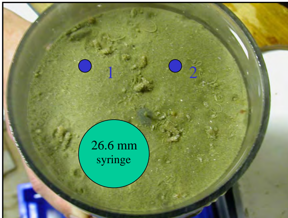
Figure 2.3-2. Resistivity profiling photographs taken aboard the R/V Vantuna during the geotechnical coring effort during the Summer 2004 Geotechnical Measurement Program. These photographs depict: A) the OSU resistivity profiling device with an extruded core positioned beneath the probe; and B) a schematic representation of the resistivity core processing at sea with the blue dots indicating the approximate location of replicate resistivity profiles and the green circle showing the approximate location of the syringe sample taken for water content analysis (core diameter is 10.8 cm).
