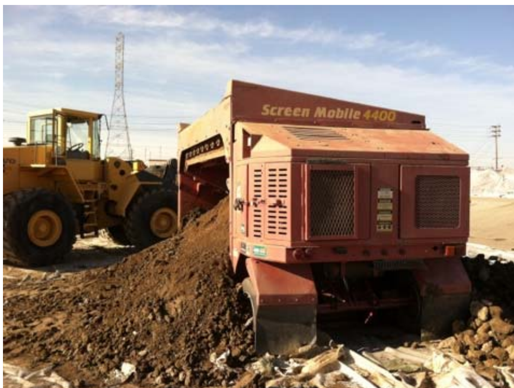
Figure 2: Soil screening machine.
