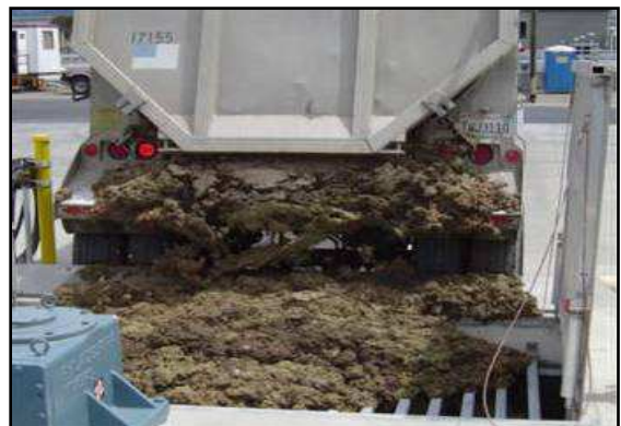
Food waste is delivered to EBMUD and screened, ground and cleaned of contaminants. A typical delivery is approximately 20 tons total weight.
