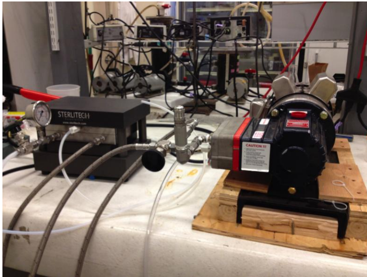
Membrane Separation Testing Unit
