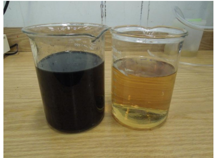
Digester Effluent before and After Filtration
