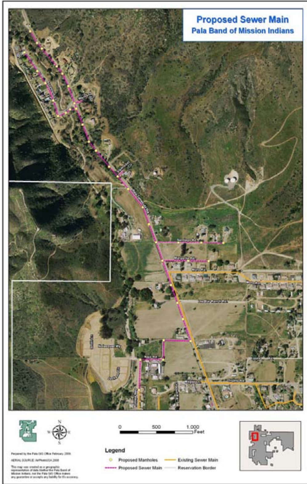
Figure 1 Proposed New Sewer Main Alignment
