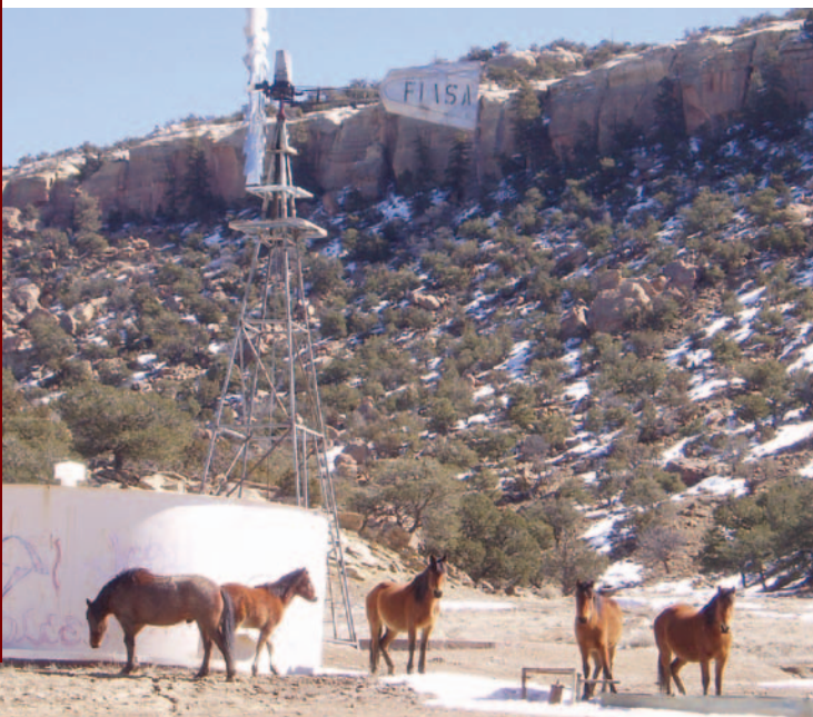
Windmill pumps groundwater into a storage tank on the Navajo Nation.
