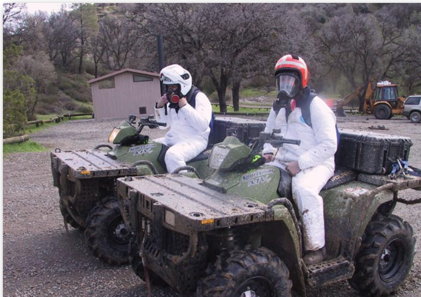
Riders with monitoring equipment and protective gear prepare to kick up asbestos-laden dust in the Clear Creek Management Area to measure what ATV enthusiasts might be breathing into their lungs.
