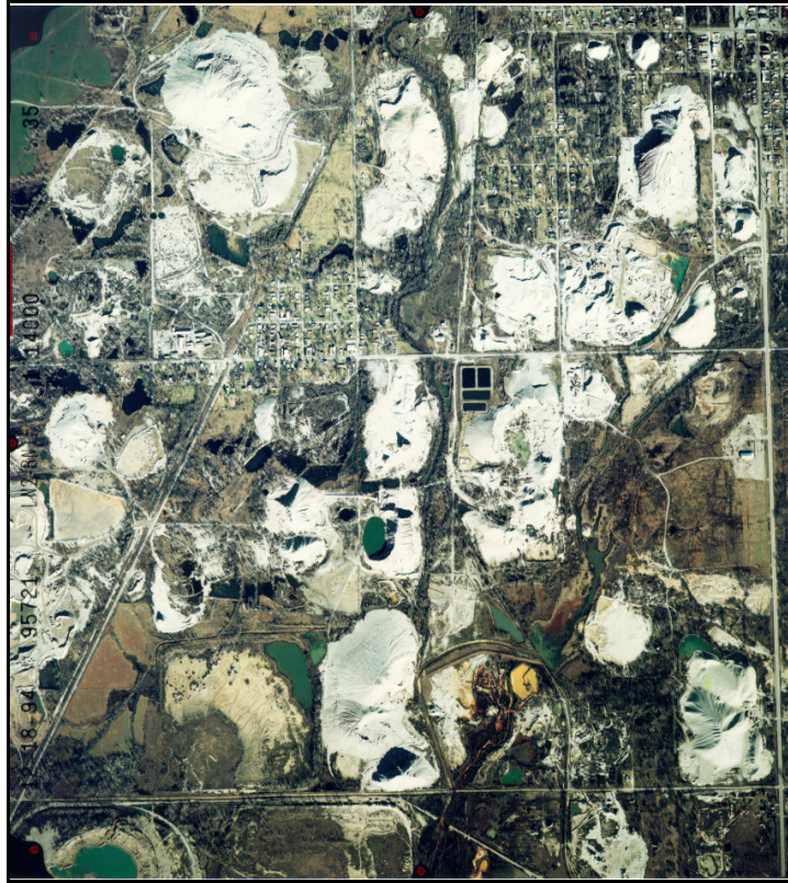
Aerial Photograph of a Portion of the Site - Note the chat piles (gray areas). Also note the acid mine discharge (yellow areas). Cardin, OK, is located in the upper left, Picher is located in the upper right.
