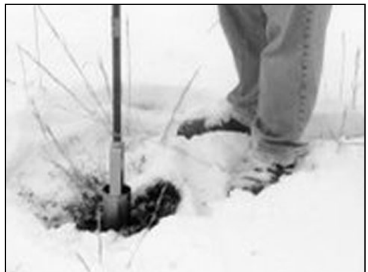
Soil sampling using a hand augur
