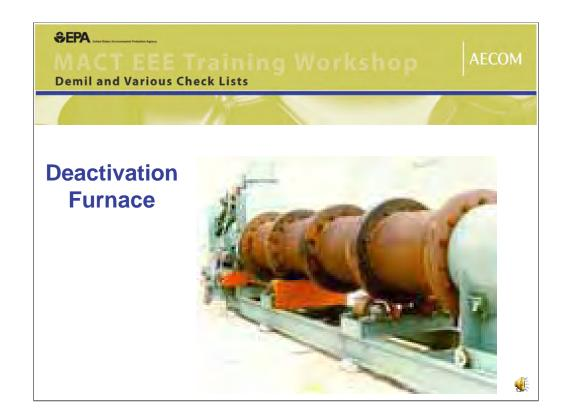
This slide shows a deactivation furnace where the propellant sections of the weapons and empty carcasses that have been drained of active agent. These component have holes in them so that an active propellant or agent can volatilize off and be combusted.
