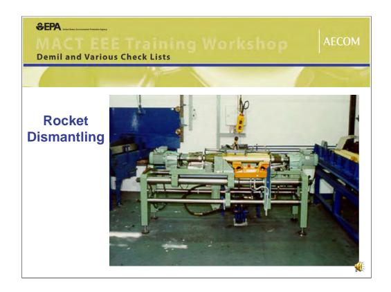
Here is a rocket dismantling unit. The purpose of this is to disassemble the warhead from the propellant so that each can be handled safely during combustion.
