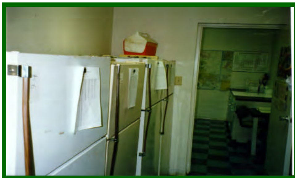
Sample storage refrigerators with identification numbers and temperature records
