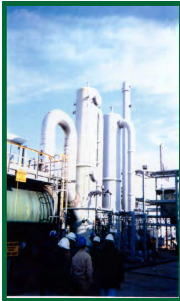
An ionizing wet scrubber used to remove HCl
