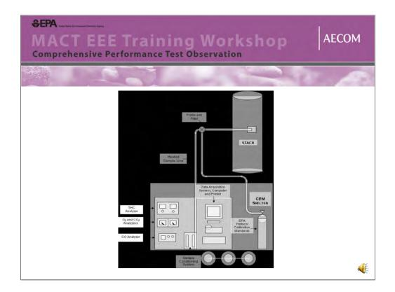
A typical portable CEMS system should look something like the schematic shown in this slide.
