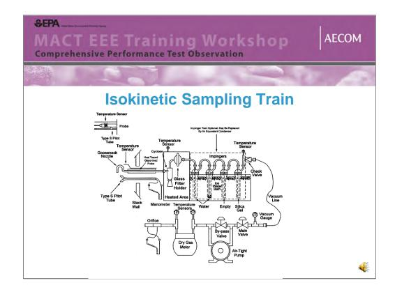
Just as a reminder, this slide shows the components of a typical isokinetic train. The number/type of impingers, their reagents and other glassware, like XAD traps for dioxin and furan analysis, will vary depending on the method.
