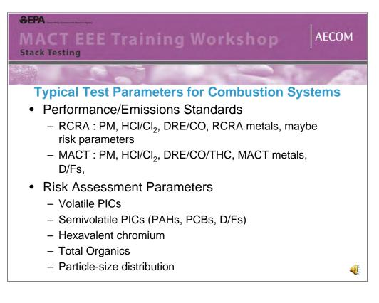
Typical test parameters for HWC units generally fall into one of two categories. Generally, they are parameters that must be evaluated for to show a unit meets the required performance/emissions standards or they are parameters that are used as input information to conduct the multi-pathway risk assessment.
