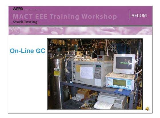
This slide shows and example of an older portable GC. Newer models are smaller and more compact.
