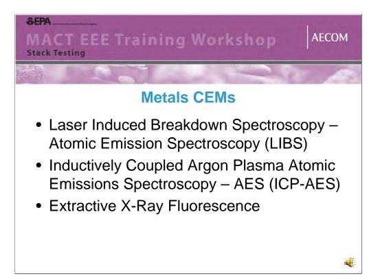
One are that has been of interest is the development of a CEMs for the continuous measurement metals in HWC emissions. Several different analyzer types have been incorporated into CEMs systems. A key issue that metals CEMs systems have to overcome, however, is collecting a representative sample of the stack gas, due in large part to the fact that metals are present as both particulate and as a vapor, making extractive sampling systems a challenge.
