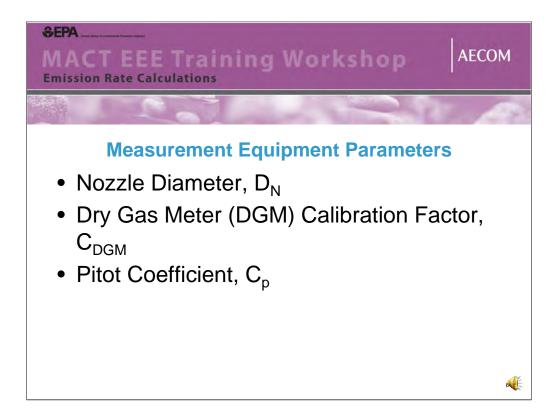
Several parameters are dependent on the sampling equipment used. The nozzle diameter, dry gas meter calibration factor and pitot tube coefficient are parameters that are based on the equipment used during a specific test.
