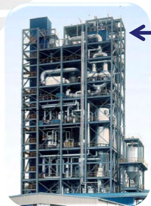
Traditional: Vertical Reactor (700 MT/day max)
