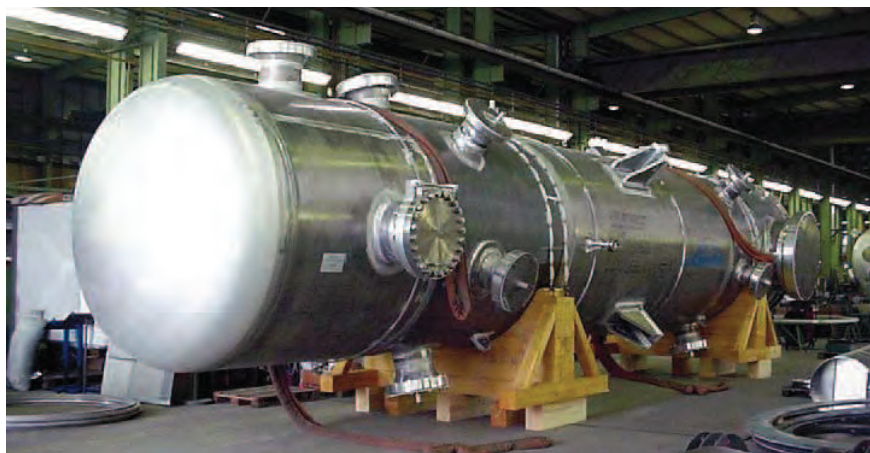
Coil-wound heat exchanger for the Stavanger LNG plant at Linde's own workshop in Schalchen, Germany
