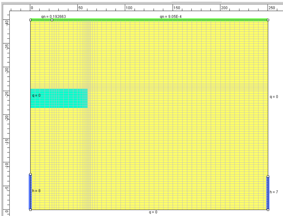
Figure 4.16. Two-dimensional unsaturated zone grid, material zones, and boundary conditions for two-dimensional unsaturated zone flow model. The grid represents a vertical profile perpendicular to the long-axis of the TWIS. Green line = ground surface with the TWIS infiltration gallery on the left between two small white squares; light blue area = low permeability unit; dark blue lines = constant-head boundary conditions to simulate 1 m drop in head ( h = 8 to h = 7 ) over the 250-m horizontal distance. Q = 0 are no-flow boundaries above the water table. The water table is at the bottom of the grid. Horizontal and vertical measurements are in meters.
