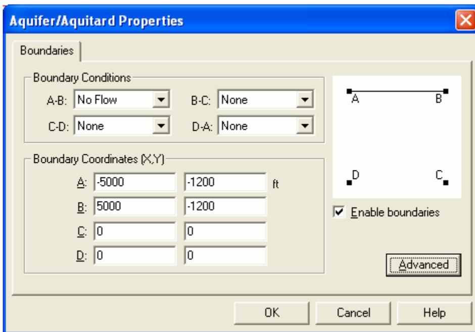
Placement of no-flow boundary. (Menu from AQTESOLV).
