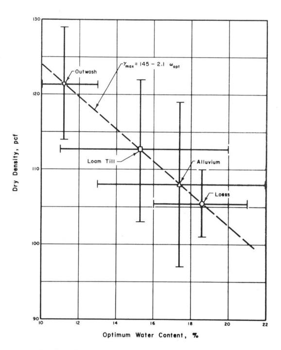
FIGURE 13. MOISTURE-DENSITY RELATIONS FOR PARENT MATERIAL GROUPS, C HORIZON, AVERAGE AND 85 PERCENTILE RANGES
