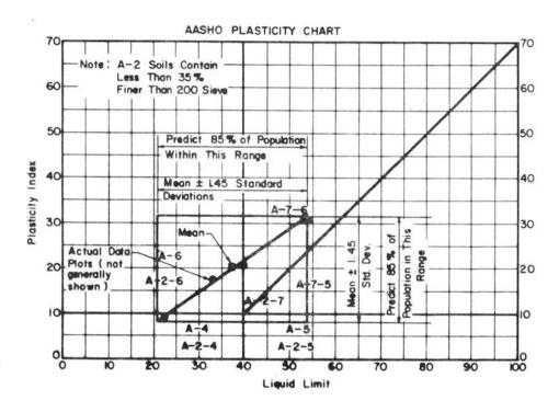
FIGURE 11. METHOD OF GRAPHICAL PRESENTATION OF MEAN AND 85 PERCENTILE RANGE FOR PLASTICITY DATA (HENNEPIN GRAVELLY LOAM, C HORIZON)
