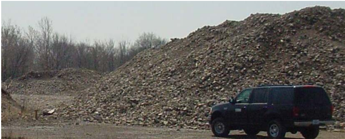
Crushed concrete stockpiles in Main Plant Area.
