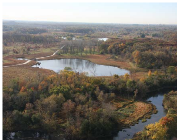
The hydric soil and gravel materials used in the restored river (lower right) were excavated from the NOAA Sanctuary Pond NOAA project (in background).
