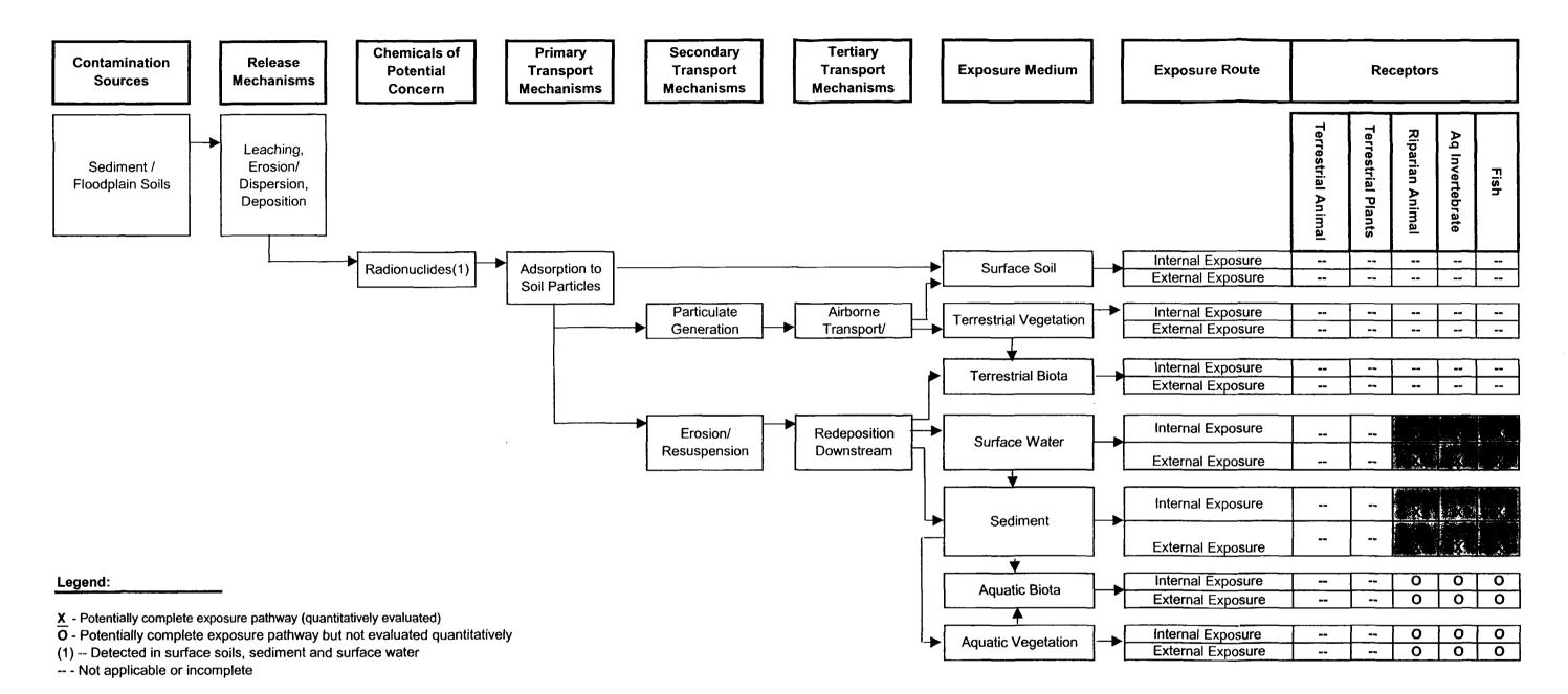
Figure 3-4. Conceptual Site Model for Chemical Contaminants
