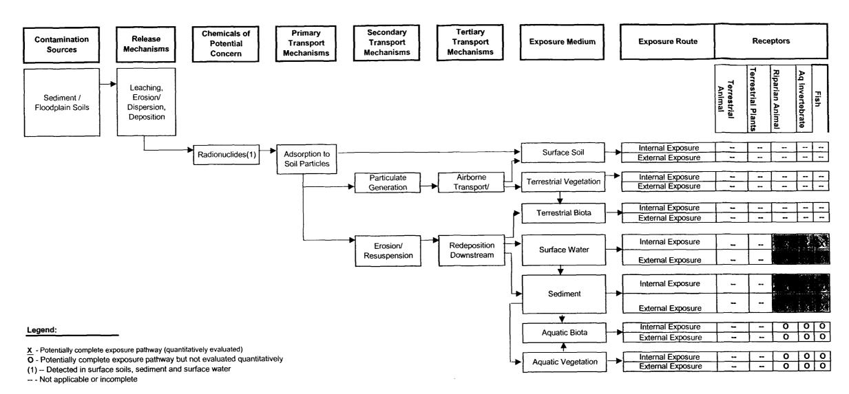
Figure 3-6. Conceptual Site Model for Chemical Contaminants
