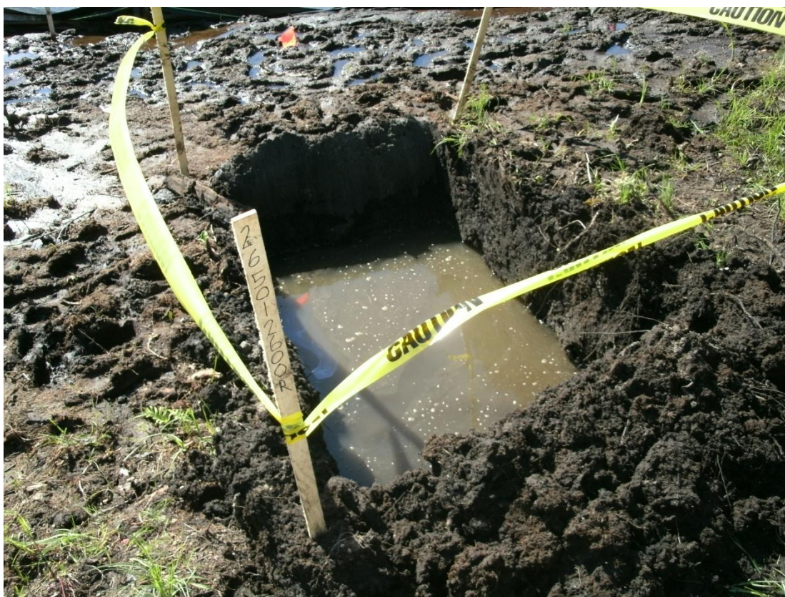
26+00R – 26+50R: Looking toward Talmadge Creek at 6-hour test pit (September 12, 2010)
