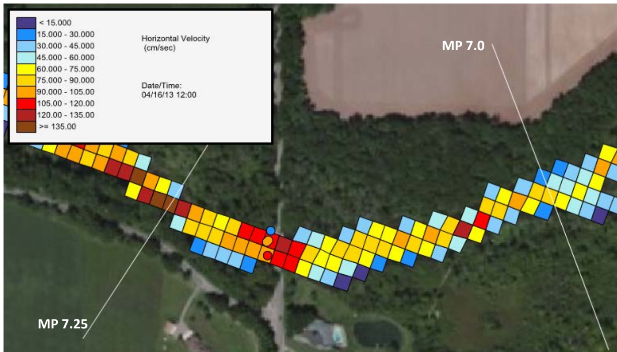
Figure B-2. Model comparison to velocity data at transect 7.18 on April 16, 2013. Circles represent velocity measurements, with transect data averaged by grid cell. Legend in 15 cm/sec increments.
