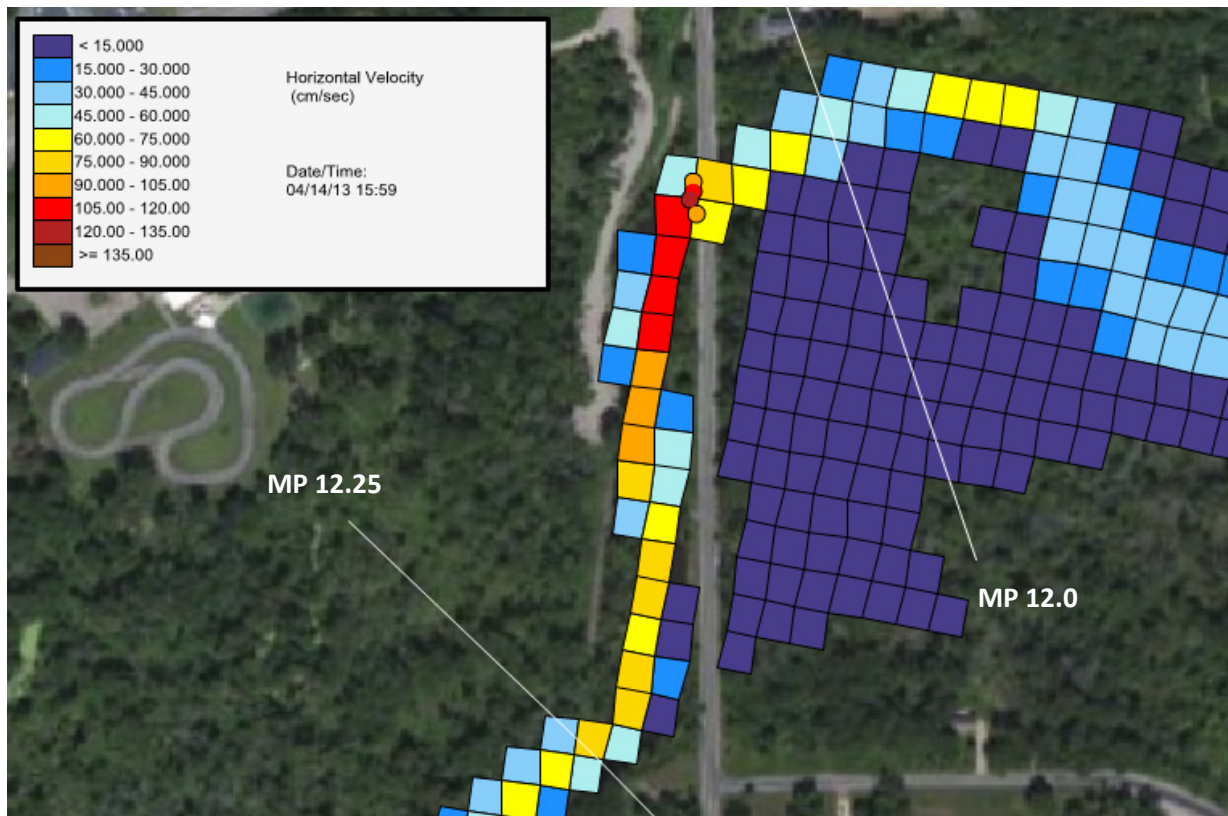
Figure B-3. Model comparison to velocity data at transect 12.05 on April 13, 2013. Circles represent velocity measurements, with transect data averaged by grid cell. Legend in 15 cm/sec increments.
