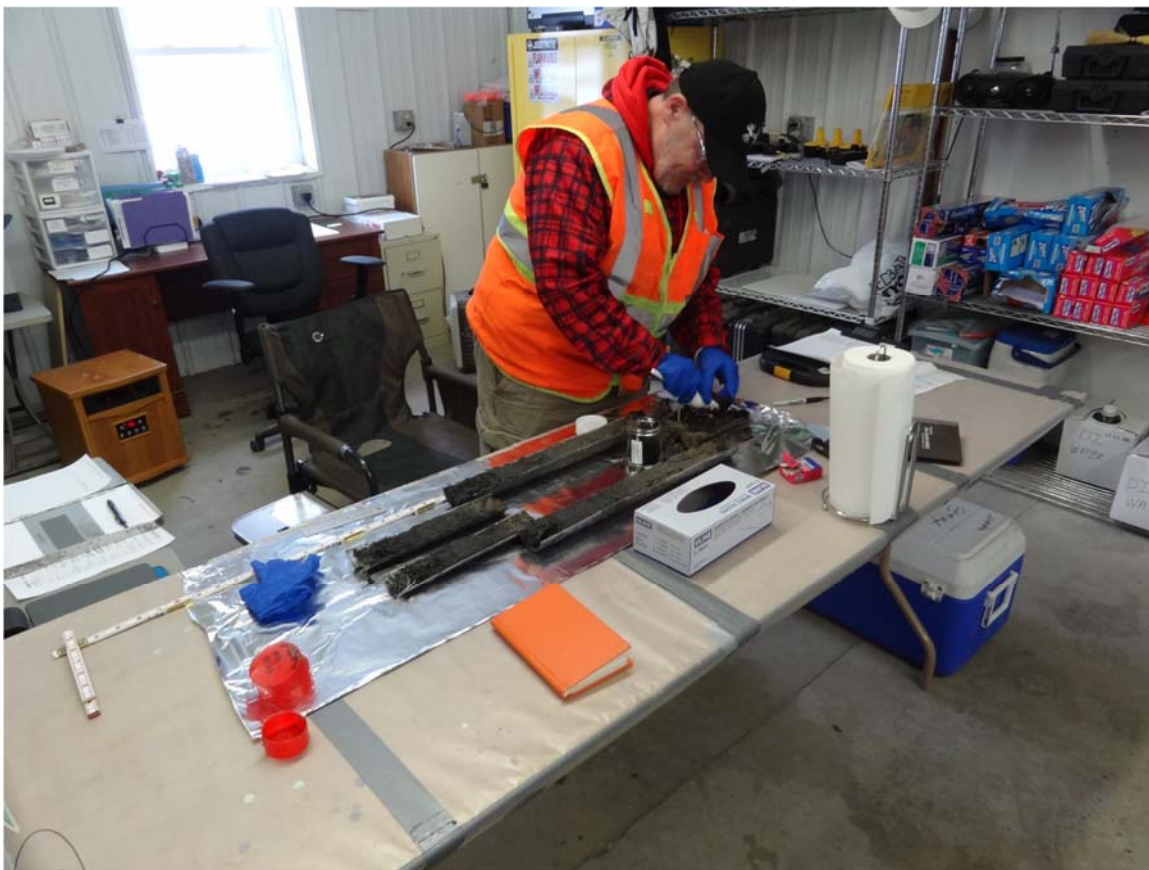
7. C3.2 Pole Barn observed core logging operations.
