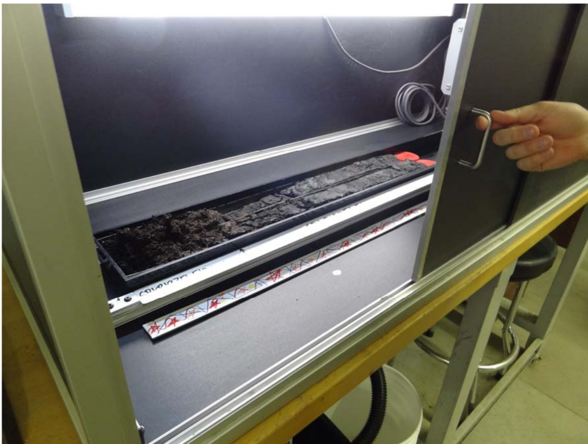
6. C3.2 Pole Barn observed core logging operations.
