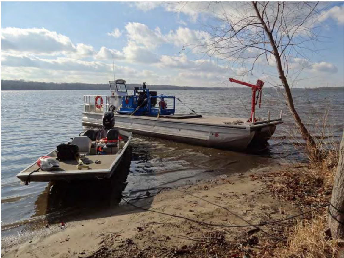
18. Pontoon boat for boom anchor removal unloaded and staged at E4.0 boat launch.
