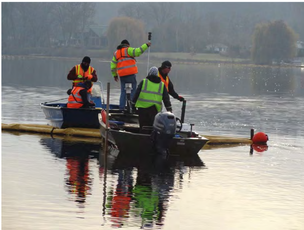
16. Post-curtain removal bathymetry crew working along boom E in west end of Morrow Lake Delta.
