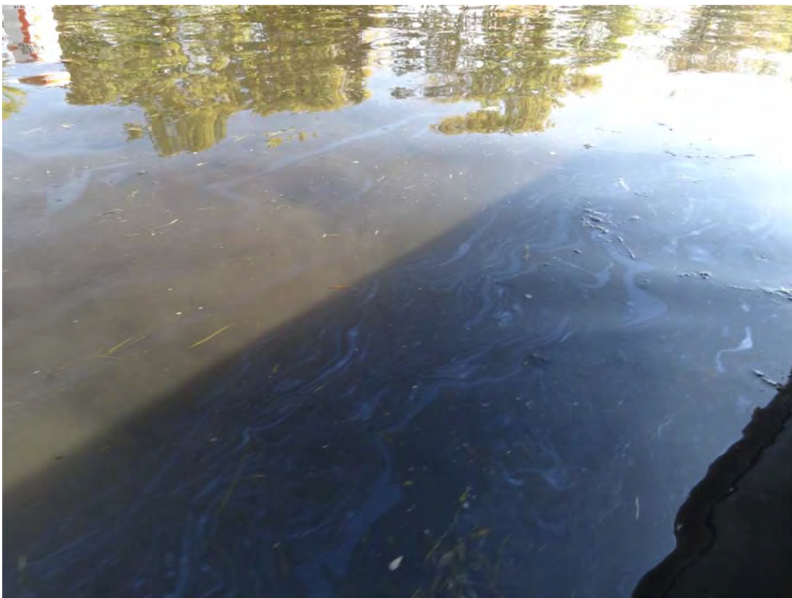
4. Sheen and tar globules observed within containment along Ceresco Dam control point.
