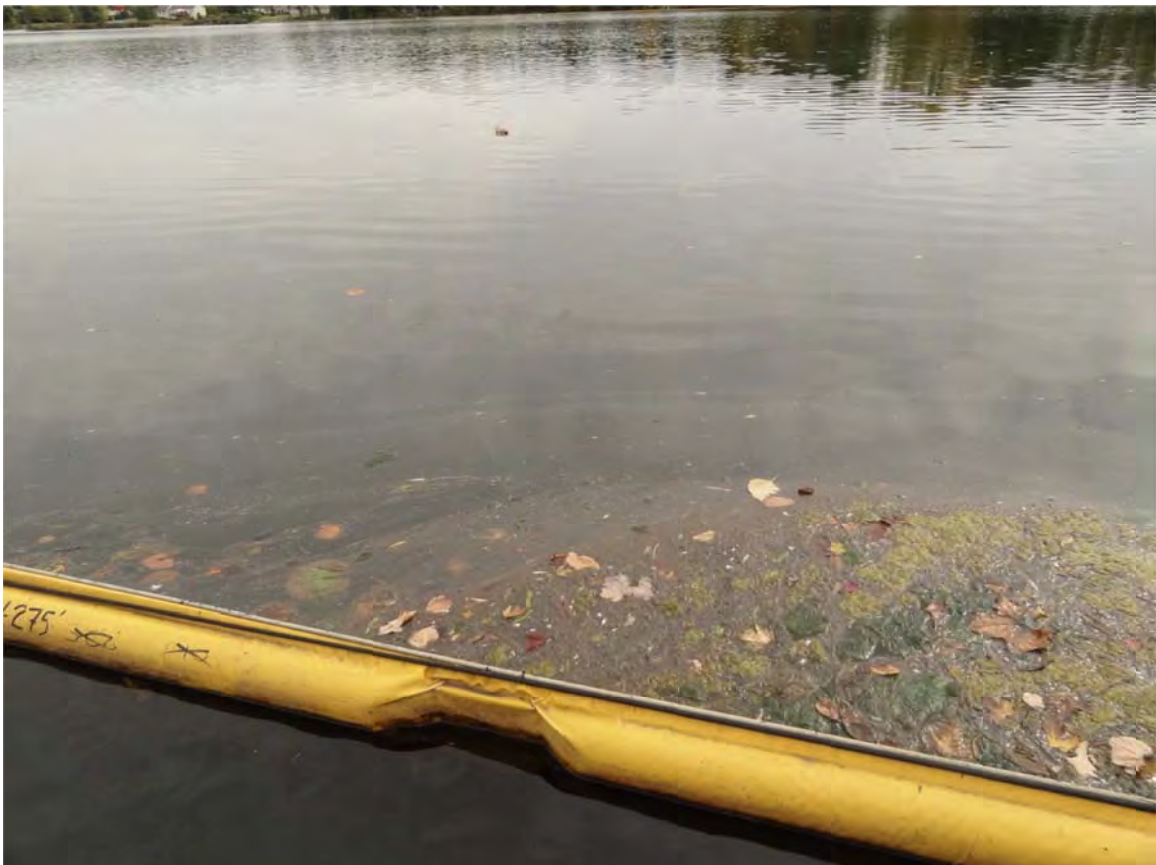
12. Boom configuration C in Morrow Lake Delta. Sheen observed along containment boom.
