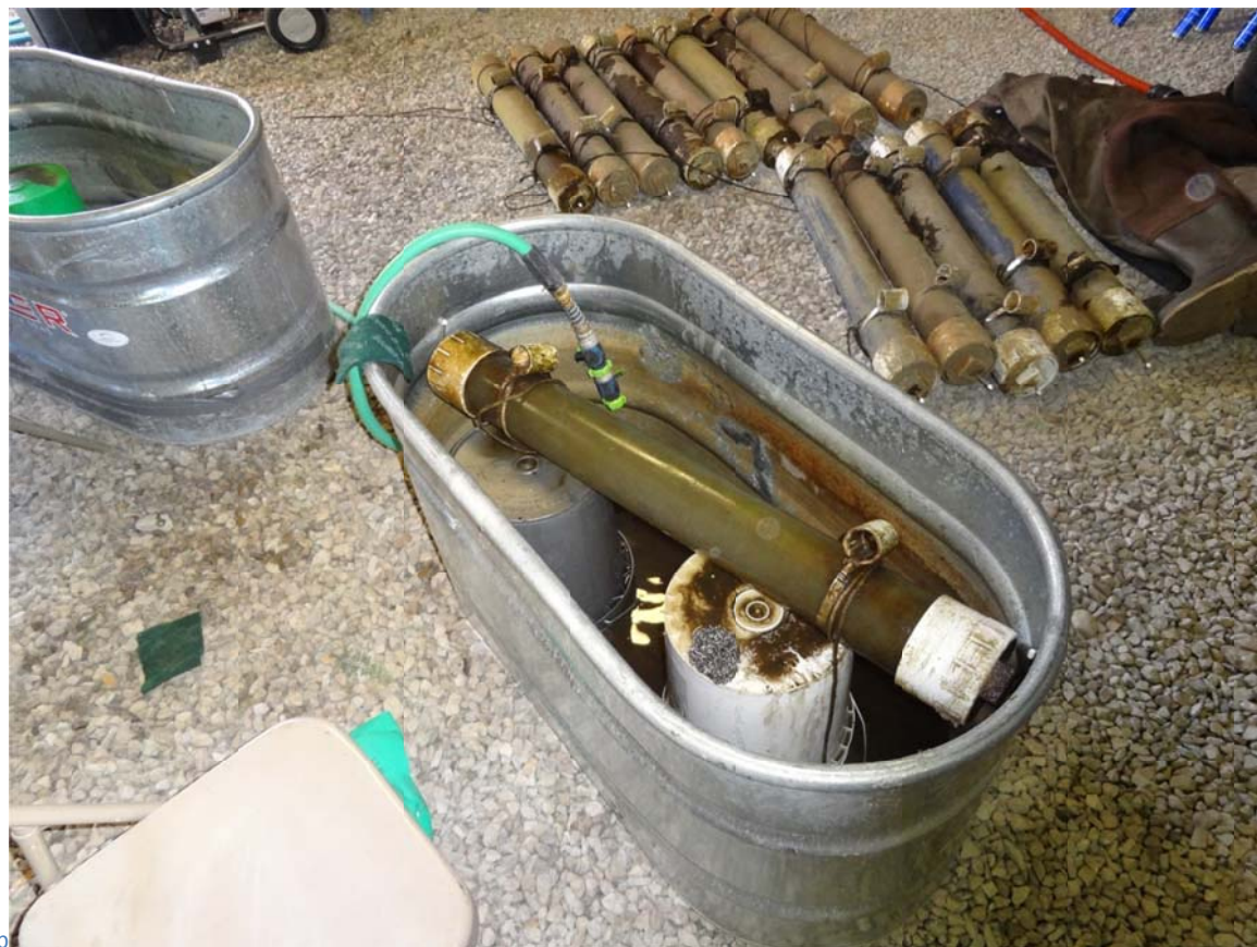
7. Walling Tube sampling observed within the barn at the C3.2 boat launch.
