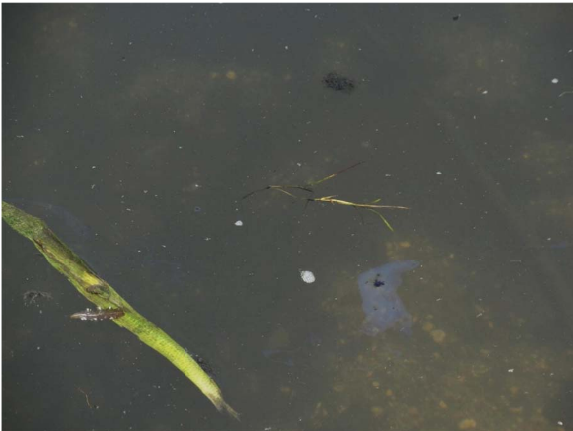
32. Portage launch below Ceresco Dam, tar globs and sheen observed. The quantity of sheen did not meet the requirements for a sheen sweep boat.
