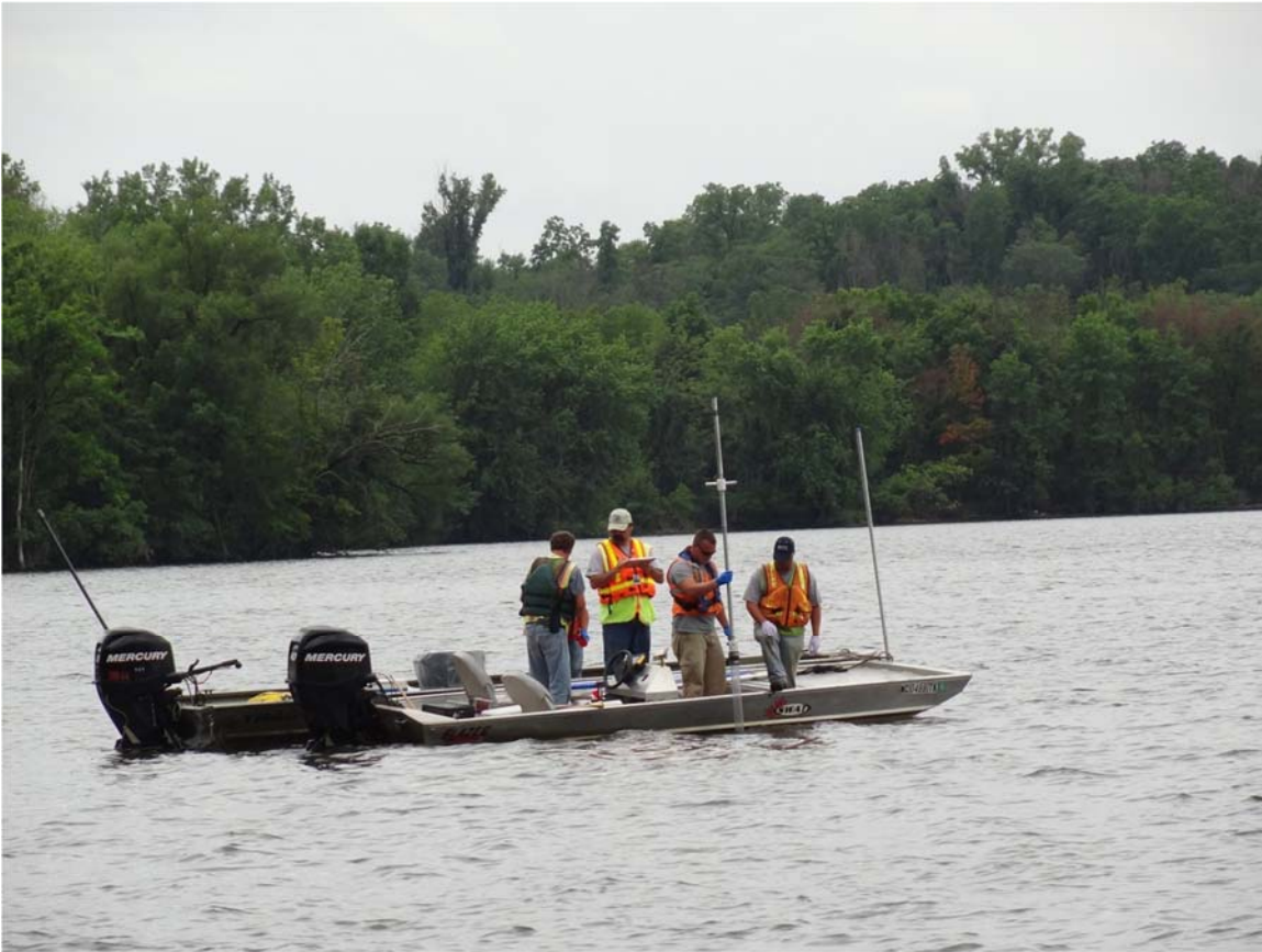
17. Morrow Lake observed quantification coring work.
