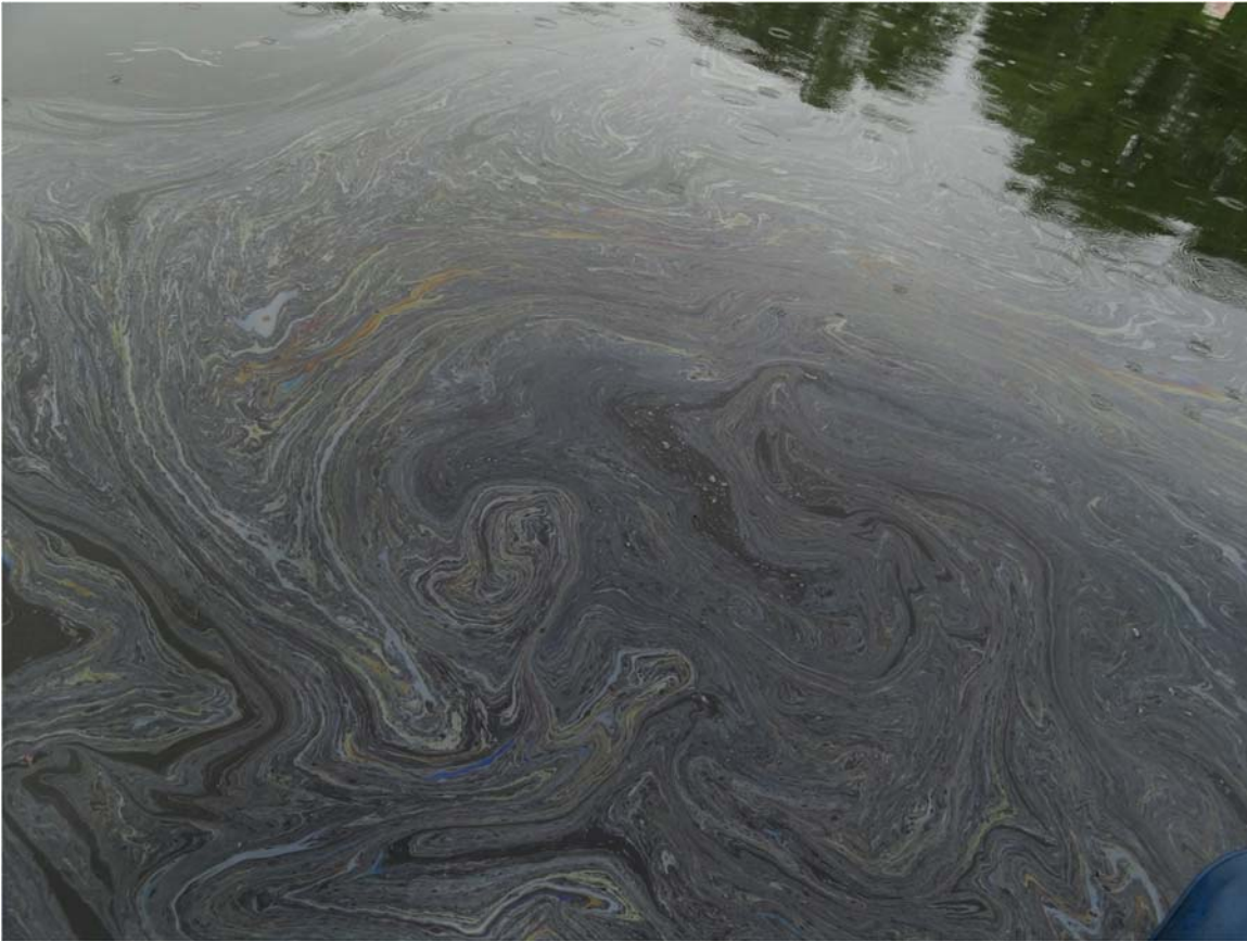
7. Ceresco Dam sheen observed when the boat agitated the sediment.
