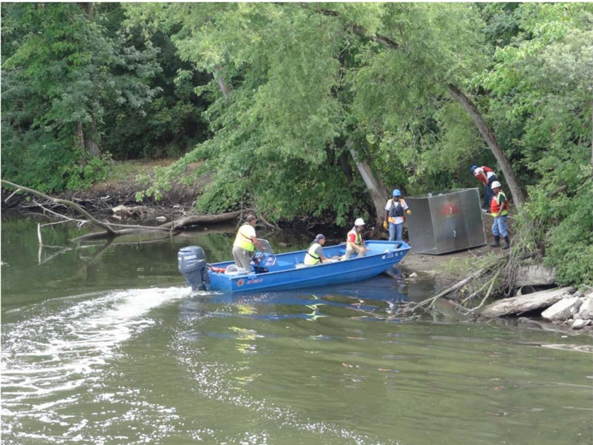
32. MP21.5 observed crew preparing to deploy the agitation affects study box.
