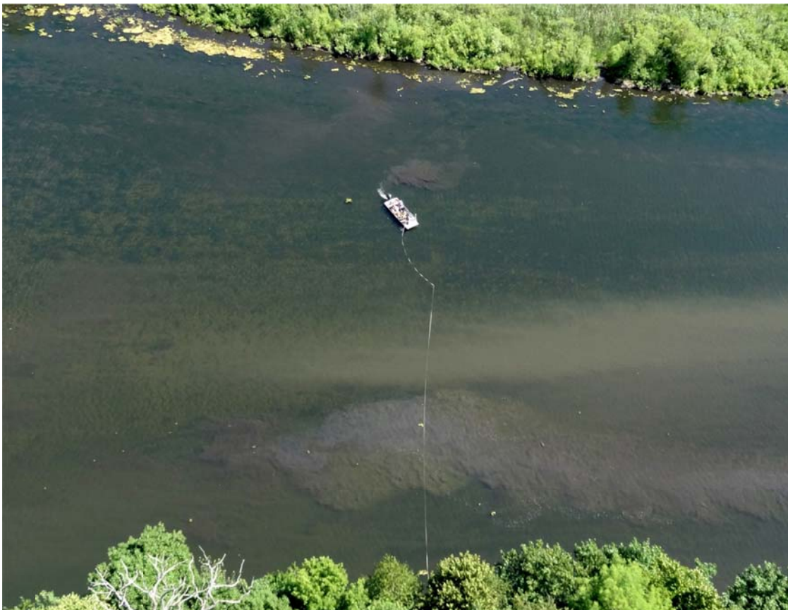
4. River velocity measurement crew measuring transect near MP5.4.
