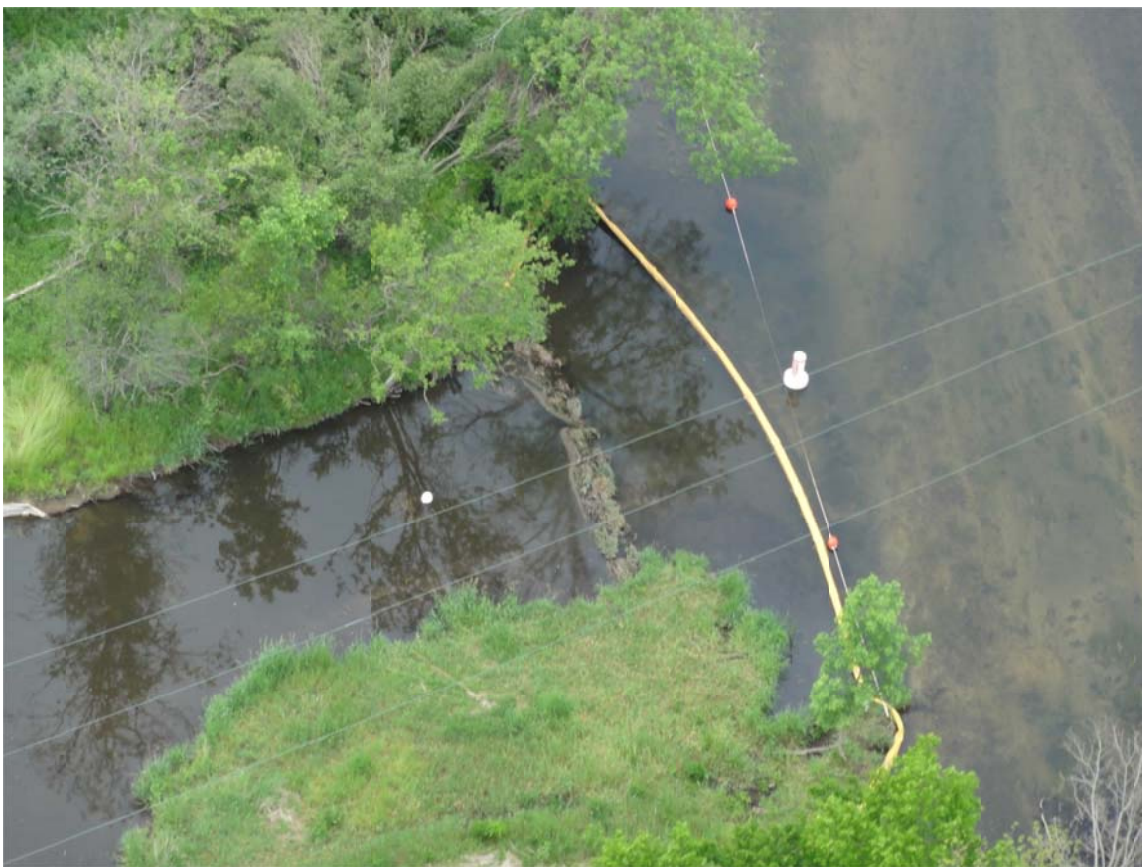
8. MP 10.75 sediment trap, sheen observed within containment.
