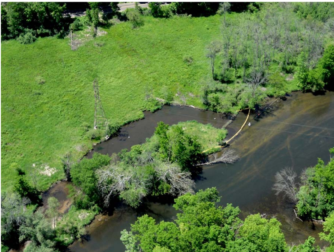
12. MP 10.75 sediment trap, sheen observed within containment.
