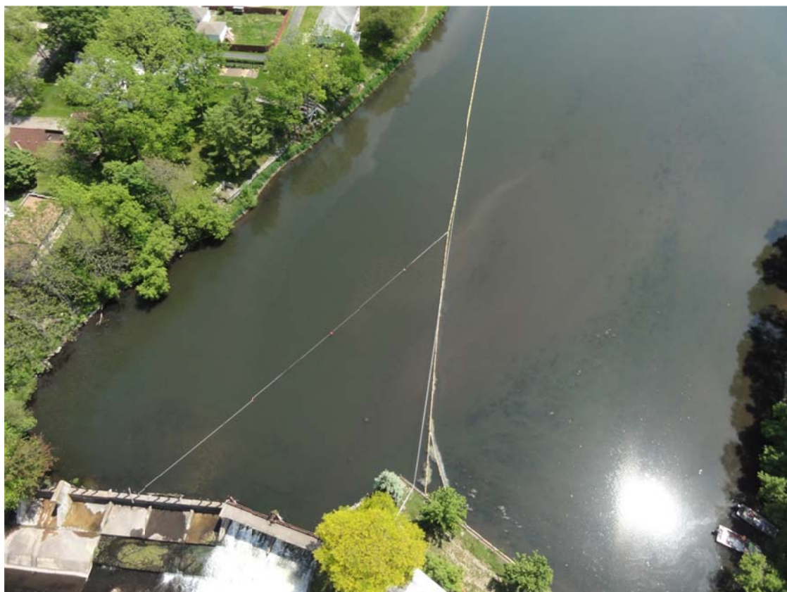
8. Control point above Ceresco Dam, sheen and some debris observed within containment.
